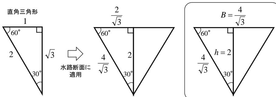
流水断面積  $A$   $A = (B \times h) \times \frac{1}{2} = \left(\frac{4}{\sqrt{3}} \times 2.0\right) \times \frac{1}{2} = 2.31\text{m}^2$
